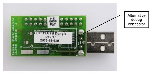
Figure 12: CC2511 Dongle back view
